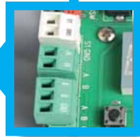
Color coded terminals for easier connections and diagnoses
